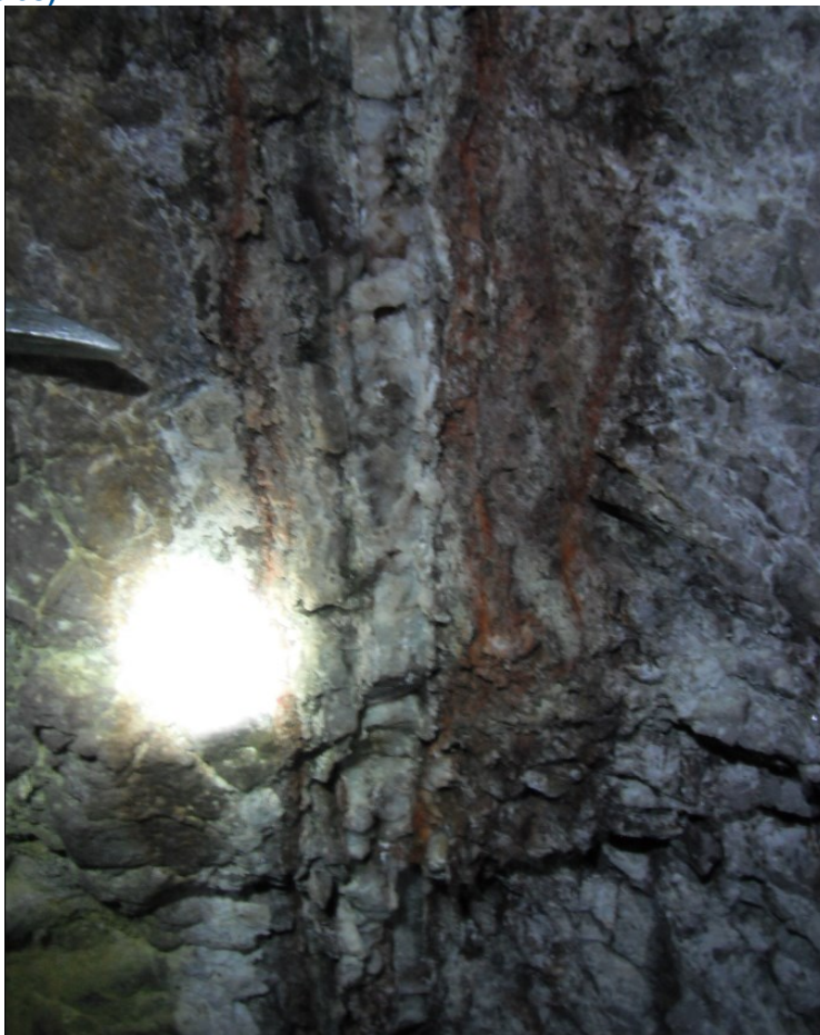
Photo 6-1: Laminated (banded) Vein Style Mineralization along Las Chispas Vein, tip of Rock Hammer shown on Upper Left (near SilverCrest sample 227908, 1.04 gpt Au and 197 gpt Ag over 1.33 metres)
