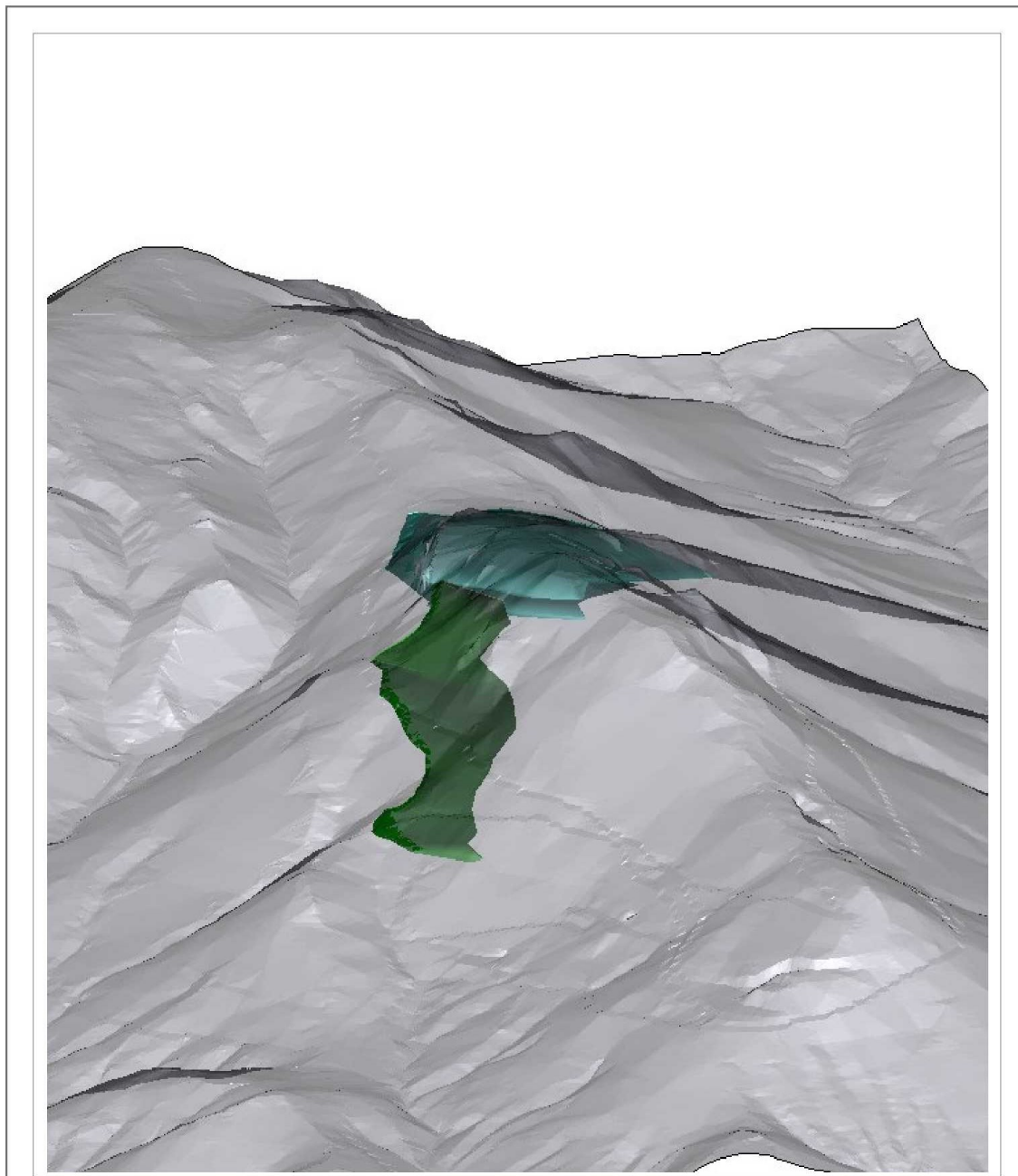
Figure 14.3: Mineralized Wireframes for East-Dipping Mineralization used to Constrain the Block Model
