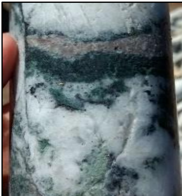
Photo 7-17: Drill Hole GR17-04; from 133.8 to 134.3 m, 0.5 m Grading 47.5 gpt Au and 5,620 gpt Ag, with Coarse Argentite, Sphalerite and Galena
