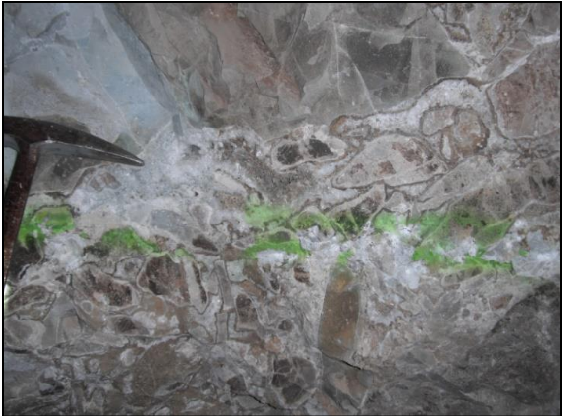
Photo 7-4: Breccia Style Mineralization Along Las Chispas Vein (Base of Las Chispas Gallery Near Silver Crest Sample 617179, 2.34 gpt Au and 344 gpt Ag)
