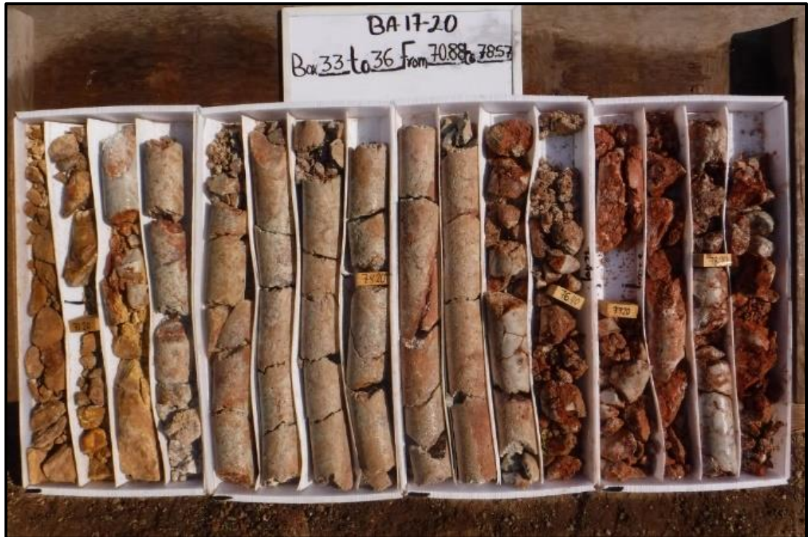
Photo 7-18: Drill Hole BA17-20, from 75.7 to 78.2 m Grading 3.05 gpt Au and, 77.8 gpt Ag
