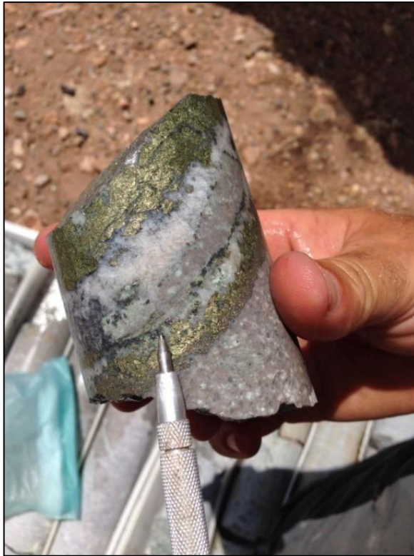
Photo 7-16: Drill Hole GR17-02; from 139.85 to 140.55 m, 0.7 m Grading 8.15 gpt Au and 387 gpt Ag, and 1.02% Cu with Coarse Argentite, Pyrite and Chalcopyrite
