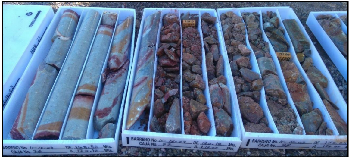
Photo 7-15: William Tell Vein, Drill Hole LC16-03, from 172 to 176 m, 4 m (1.5 m True Width) Grading 2.03 gpt Au and 683 gpt Ag
